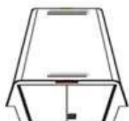
LED Lighting Option B 20" Rear Light 20" Front Light
