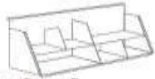
❑ Option P Horizontal Shelf Center Divider, with 1 Vertical Rear Top & 1 Forward Bottom
